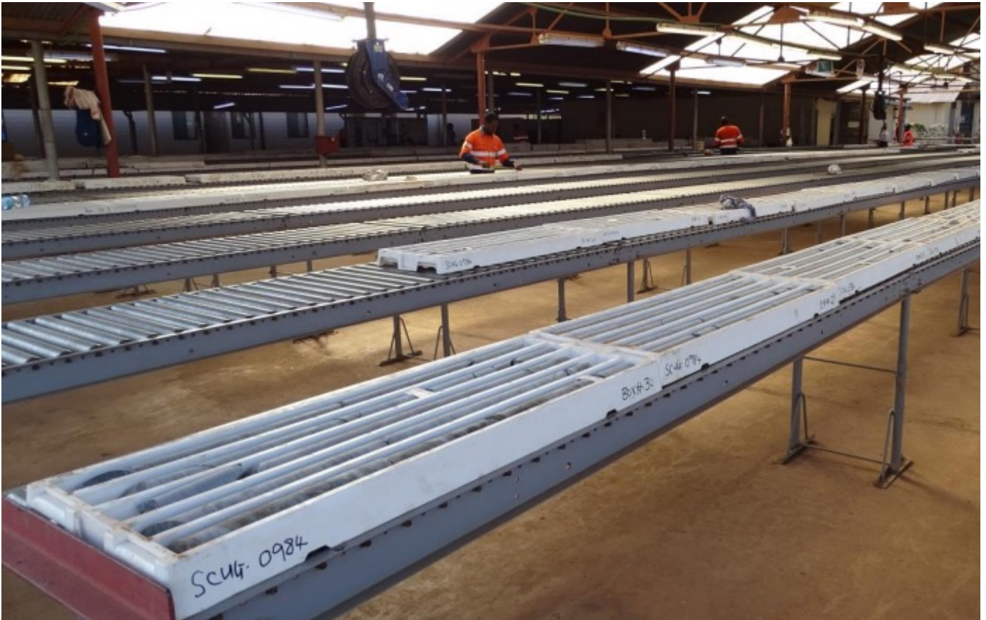
Setup of the conveyor roller racks at Core shed.
